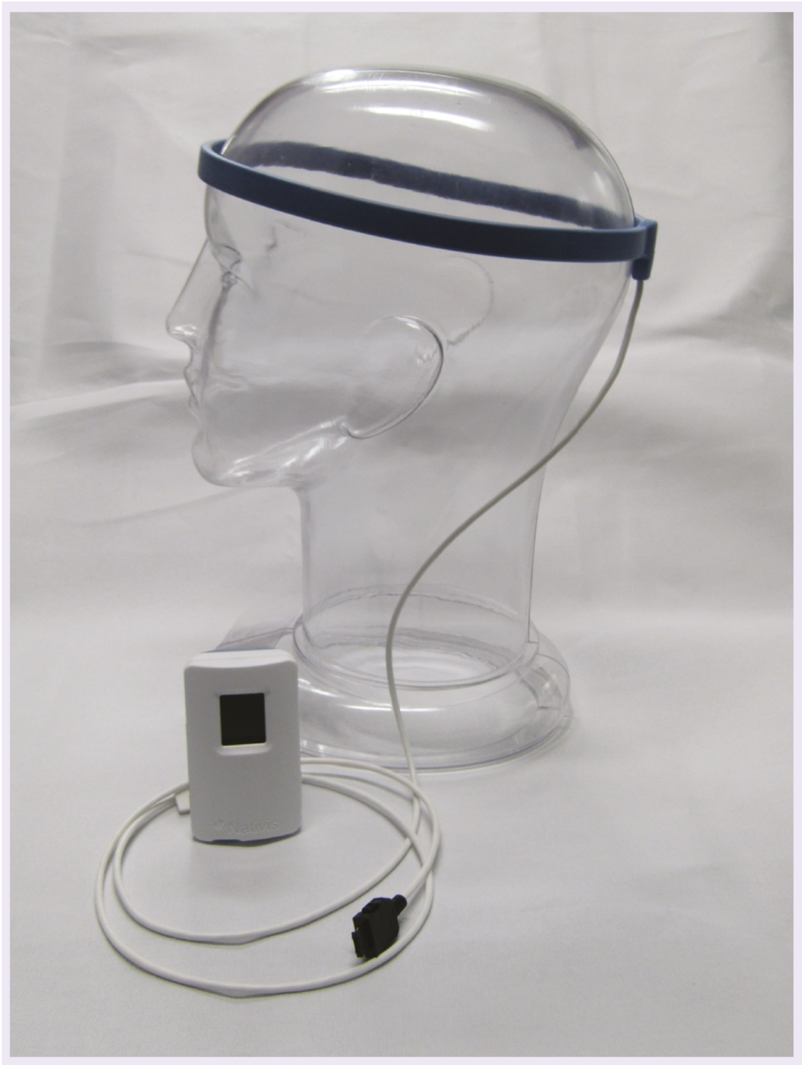
Figure 1. Nativis Voyager device as worn by a patient. The Voyager headband is placed on the patient's head and connected to the controller. It is a closed-loop solenoid coil over-molded in a medical-grade silicone designed to generate a nonlinear and oscillating magnetic field. The flexible headband is available in four sizes and includes a 2-conductor cable with a latching connector for the Voyager controller, which weighs only 2.7 ounces and is approximately the size of a pager. The Voyager controller is clipped to the patient's pocket, belt or armband. It is a software-controlled amplifier powered by a rechargeable lithium-ion battery that delivers a cognate to the patient via the Voyager headband. The small, lightweight device includes a single recessed power button and an liquid crystal display that enables the user to read the device status. There is no user-programming required, and there is no personal health information stored within the device. The device does not require the patient to shave his or her head or any other special preparation for use. Reproduced with permission from [9].
