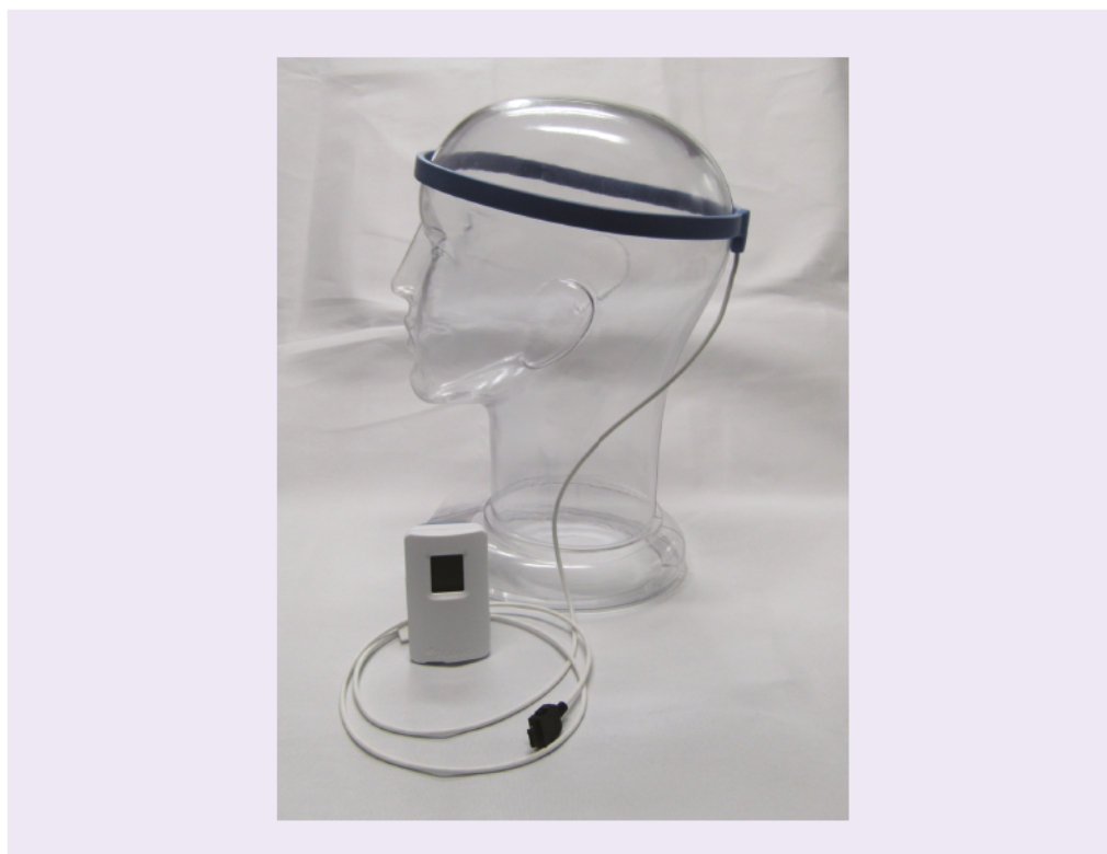
Figure 1. Nativis Voyager device as worn by a patient. The Voyager headband is placed on the patient's head and connected to the controller. It is a closed-loop solenoid coil overmolded in a medical-grade silicone designed to generate a nonlinear, oscillating magnetic field. The flexible headband is available in four sizes and includes a two-conductor cable with a latching connector for the Voyager controller. The Voyager controller is clipped to the patient's pocket, belt or armband. It is a software-controlled amplifier powered by a rechargeable lithium-ion battery that delivers a cognate to the patient via the Voyager headband. The small, lightweight, device includes a single recessed power button and an LCD display that enables the user to read the device status. There is no user-programming required and there is no personal health information stored within the device.
