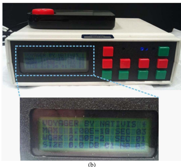
Figure S5. Signal delivery for taxane signal. (a) Diagrammatic representation of signal delivery set up and components. Numbers 568 and 570 represent the optical path for the spectrophotometer. Numbers 553 - 558 are integral components of the Voyager VX unit; (b) Prototype system with integral electronics and amplifier: Voyager VX (inset, LCD unit display of power settings).
